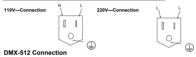
The fixture is equipped with 5 pin XLR cable mounted sockets for DMX input and output. The sockets are wired in parallel. Only use a shielded twisted pair cable designed for RS-485 and 5 pin XLR plugs and connectors in order to connect the controller with the fixture or the fixture with another.
