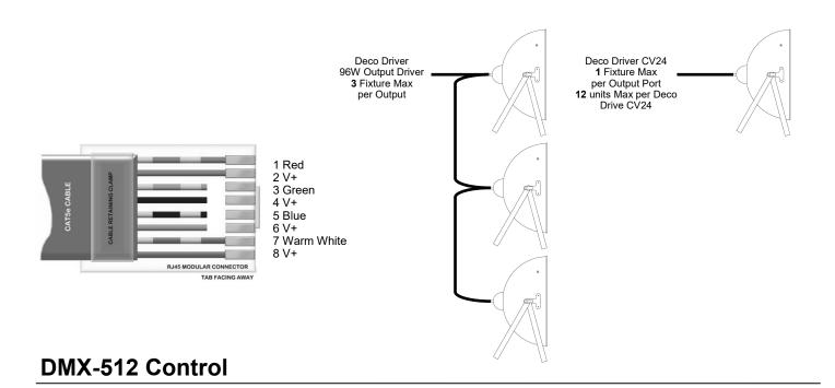
When using the Deco Vintage Scoop Q32 with Deco Drivers the fixture is intended to be used in Ch4 or Ch7 modes. The Deco Driver will be required to be set in Ch4 or Ch7 operating modes.
